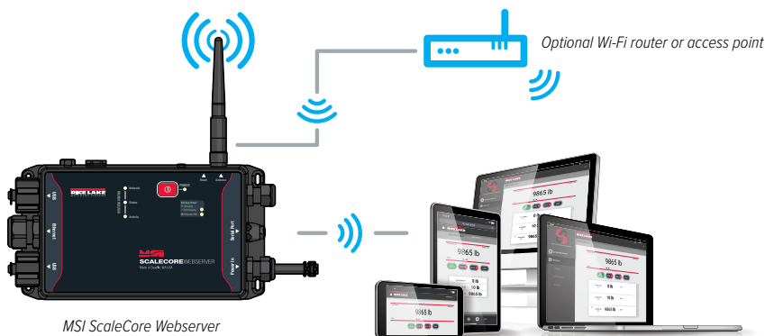
Display multiple ScaleCore devices using a web browser
