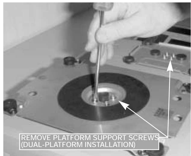
Figure 2-6. Removing Platter Support Screws and Platter Support on a Dual-Platform Scale
