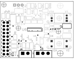
Figure 4. RS-232 Serial Fiber Optic Board
