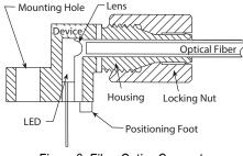
Figure 3. Fiber Optics Connector
