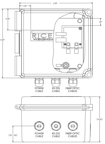
Figure 1. Fiber Optics to RS-232 FRP Converter (shown in inches)
