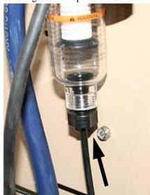
22. Guide the bottom portion of the tubing through the exit hole in the bottom of the battery box.
