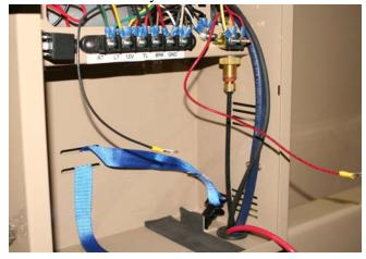
11. Remove the valve fitting by using a 9/16" wrench.
