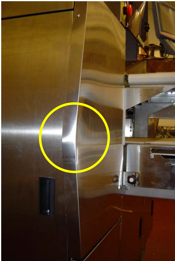
Photo 1. Damaged covers from improper strapping at mid-body.
