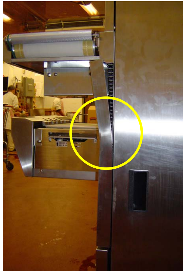
Photo 1. Damaged covers from improper strapping at mid-body.
