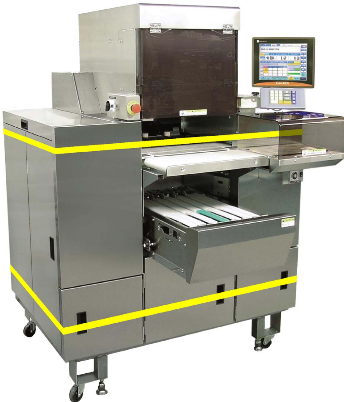
Photo 2. Correct strapping points.
