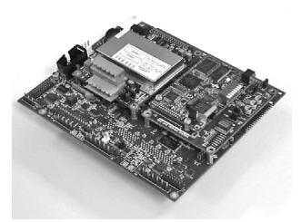
Figure 2-2. Option Installed on 920i CPU Board
