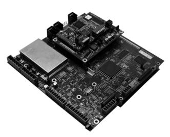
Figure 2-1. Option Installed on 820i CPU Board
