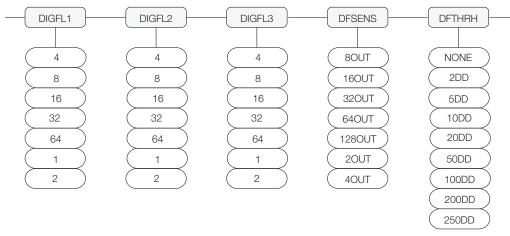
Figure 8-3. Digital Filtering Parameters on the Configuration (CONFIG) Menu
