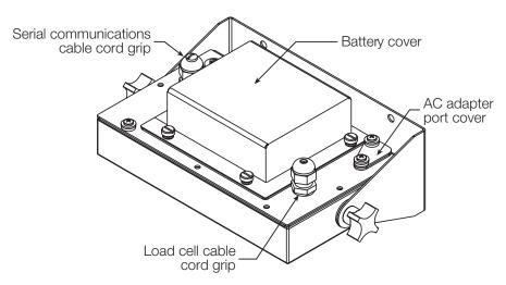
Figure 2-1. 390-DC Backplate, Showing Key Component Locations
