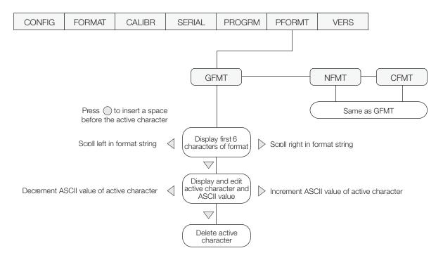
Figure 7-1. PFORMT Menu, Showing Alphanumeric Character Entry Procedure
