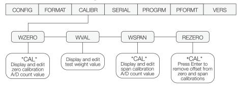
Figure 4-1. Calibration (CALIBR) Menu
