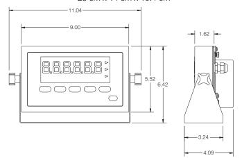
Weight Rating/Material 1.42 Kg (3.13 lb) NEMA 4X/IP66, stainless steel
