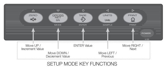
Figure 3-2. Front Panel Key Functions in Setup Mode
