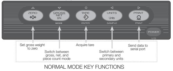
Figure 1-1. Front Panel Key Functions in Normal Mode
