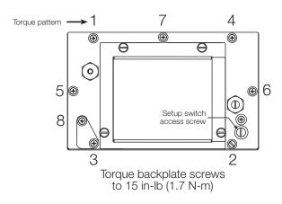
Figure 2-4. 390-DC Enclosure Backplate
