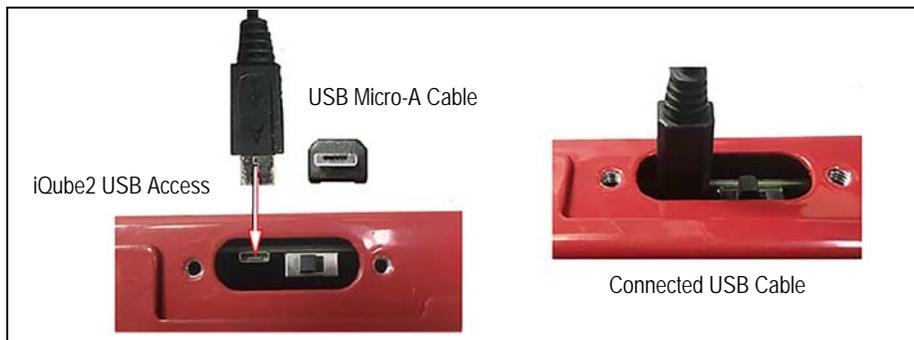
Figure 1. Firmware Update Cable Connection
