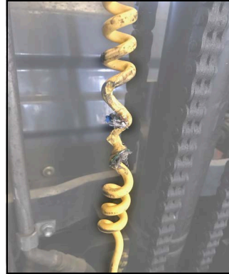
Figure 9. Detail of Damaged Cable
