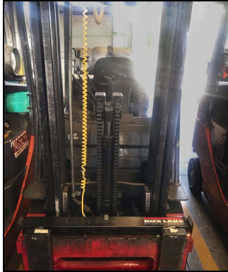
Figure 8. Inadequately Secured Coiled Cable
