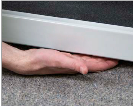
Figure 2-5. Scale Base Clearance
