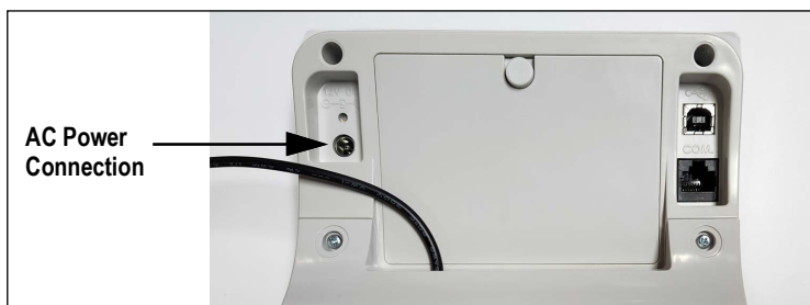
Figure 2-11. Power Connection Site
