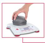
Draftshield Protects the sample from external influences, increasing the speed and repeatability of measurements
