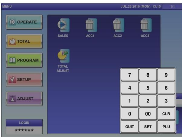
Press [ADJUST] and [LOGIN] button, then input password "495344" using numerical keys, and press [SET] button.
