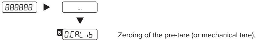
This functionality allows to zero the weigh of the scale structure (e.g. empty silo, conveyor, etc.) without changing the calibration in memory.
