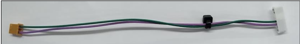
Left-Side Peel Sensor Harness C2, Old-Style Orange Connector p/n 195858 for Uni-7 s/n 100171921 to 100237827
