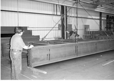
The top module can be lifted using four chains attached to the four lift lugs provided with the scale. Once the first module is removed from the truck and is placed on the setting blocks, the four lift lugs can be removed and used for lifting and positioning the other modules.
