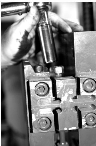
Figure 6-3. Removal of Hex Nut (#1 of Parts Breakdown)
