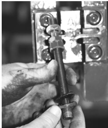
Figure 6-5. Remove Flexure Rod with Nuts and Washers
