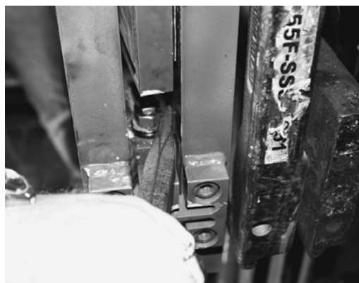
Figure 6-12. Centering the Load Cell Using a Chisel
