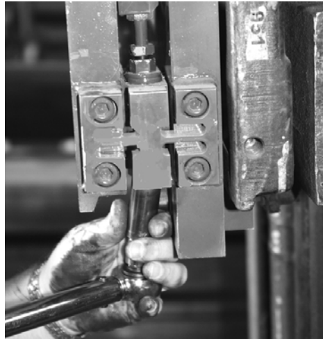
Figure 6-13. Tightening the Lower Hex Nut
