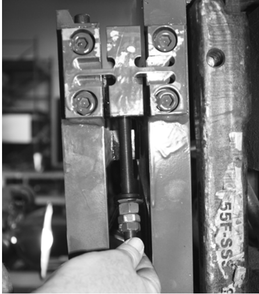
Figure 6-8. Installing Flexure into Scale
