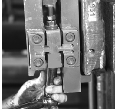
Figure 6-4. Loosen and Remove Bottom Hex Nut (#18 and #19 on Parts Breakdown)
