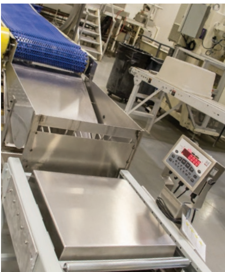
Static checkweighing with a CW90 bench scale in a pasta-producing facility requires hands-on interaction.
