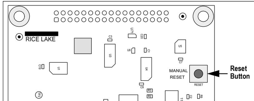
Figure 4. Reset Button Location
