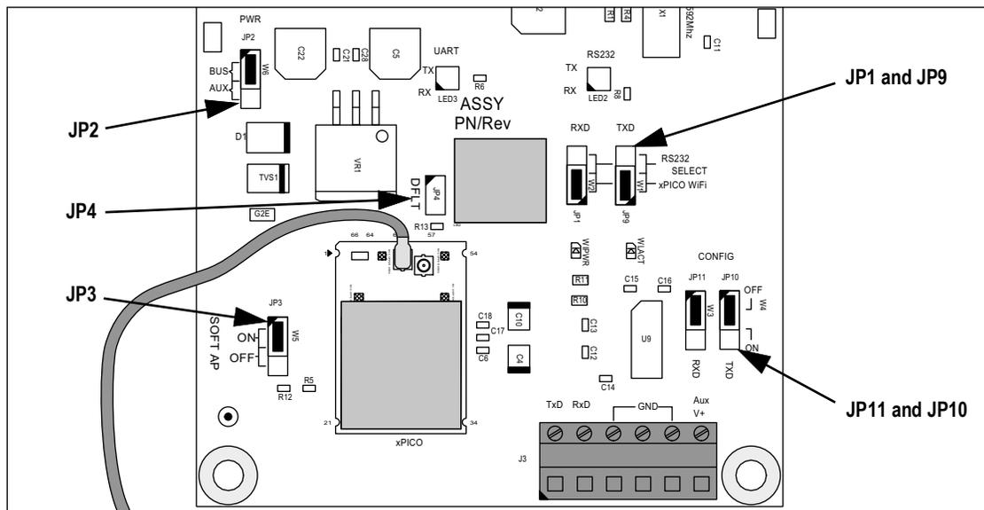
Figure 3. Jumper Locations on the WLAN Option Board
