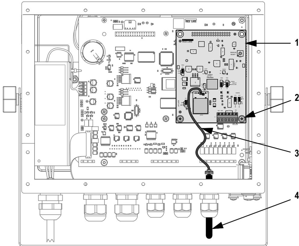
Figure 1. WLAN Option Parts Breakdown (Inside 920i Enclosure)
