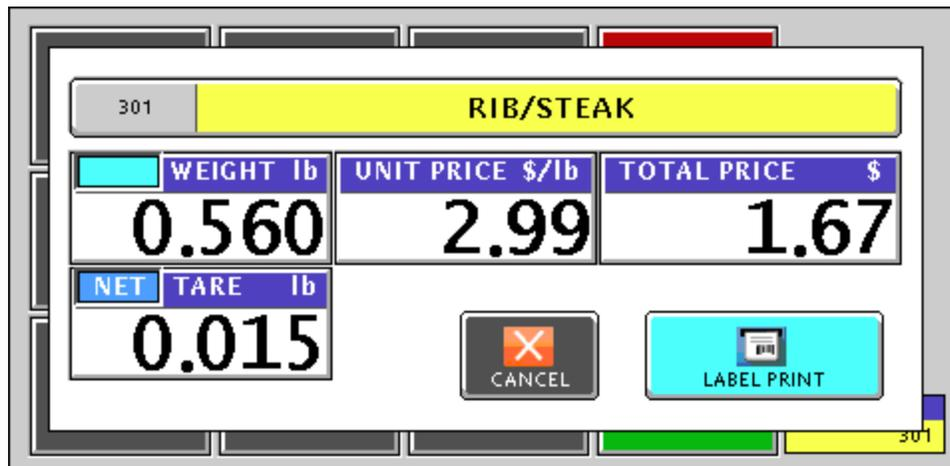
4.2 Fixed Price/Weight items: Press the LABEL PRINT button or press the CANCEL to return to the PLU selection screen. If more than one piece is purchased enter the value using the numeric keys and press the PCS field.
