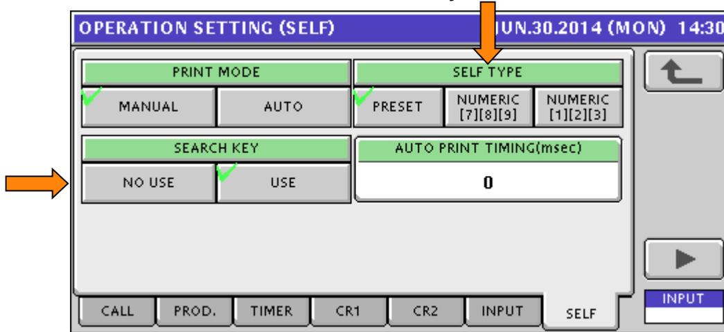
2.4 If enabled, configure Search to check the first two lines of all PLUs:
