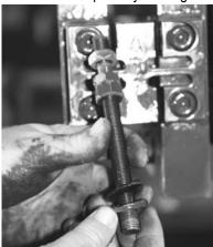
Figure 6-5. Remove Flexure Rod with Nuts and Washers
