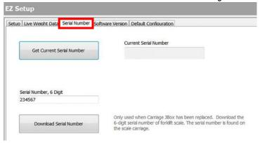
Figure 4-33. Serial Number Tab
