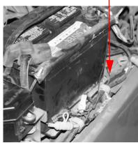
Figure 3-10. Connect Positive Wire to Battery Cable
