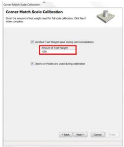
Figure 5-27. Enter Test Weight Value
