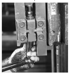
Figure 6-13. Tightening the Lower Hex Nut
