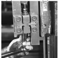
Figure 6-4. Loosen and Remove Bottom Hex Nut (#18 and #19 on Parts Breakdown)
