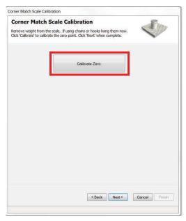
Figure 5-14. Calibrate Zero
