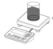
Add the third component to the container, bringing the total up to the desired target (in this example, 2000 g).
