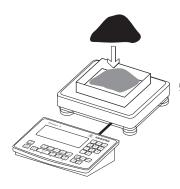
Continuing filling the container until the target amount is reached (in this example, 100%)
