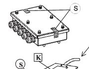
If there is a junction box between the load receptor and the electronic evaluation unit, the junction has to be secured against tampering.
