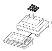
Place a number of parts in the container for the reference quantity (in this example, 10 pcs)
