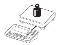
Position the calibration/adjustment weight on the weighing platform
