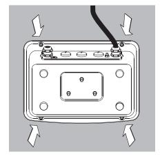
Connect the weighing platform connection cable to the indicator Note:
