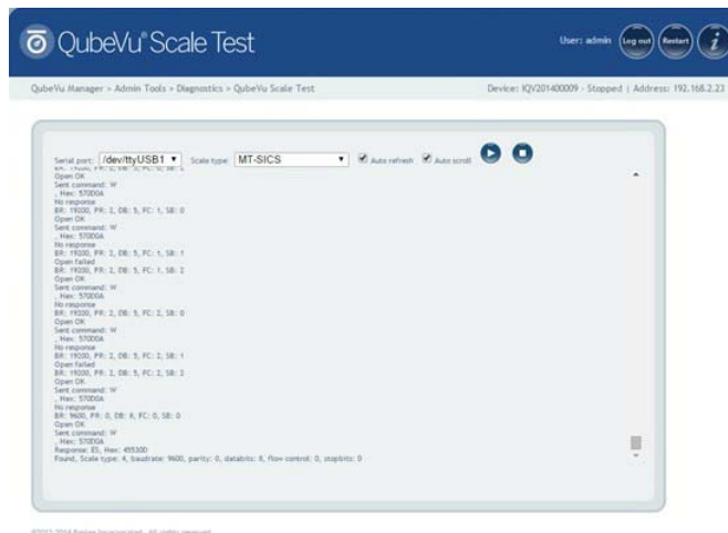
Figure 5-42. Scale Communication Parameters
