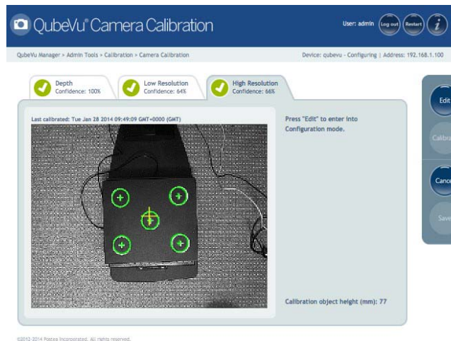
Figure 5-26. Center the Yellow Diagonal Lines on the Calibration Object
