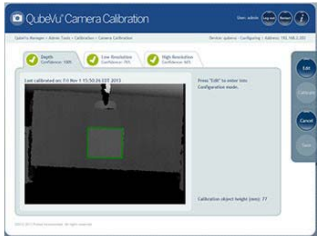
Figure 5-25. Select Edit to Start the Calibration Process
