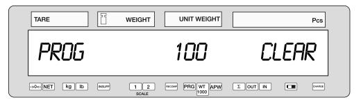
Press the **CLEAR** key to delete this Item Code and all of its data, or press the **MODE** key to cancel the deletion. If you pressed the **CLEAR** key, the Item Code will be deleted and the scale will return to the Programming Mode screen.
