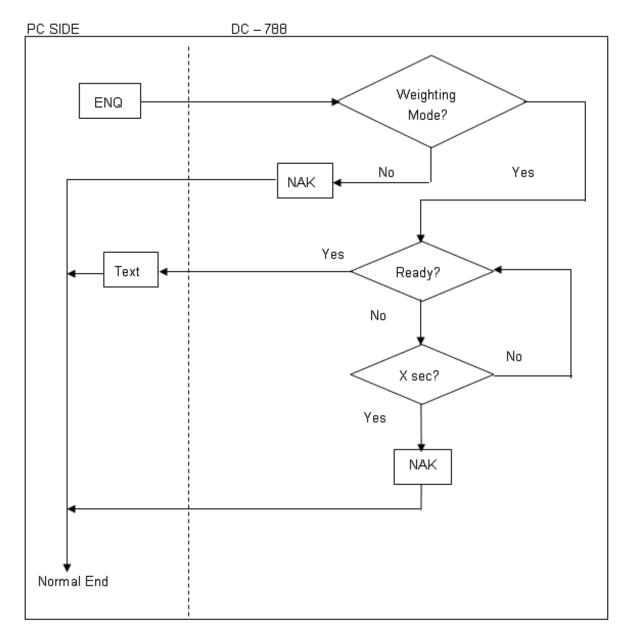
Figure 7-10. Standard Command Data Transmission Flowchart
