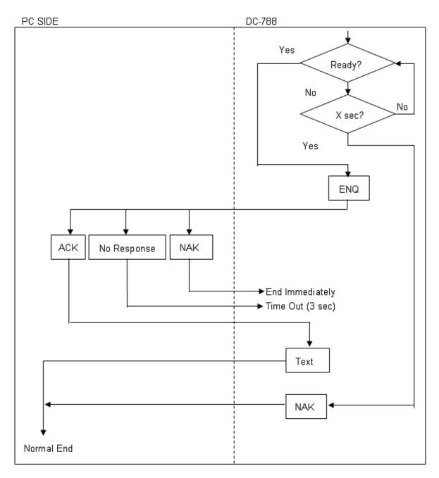
Figure 7-8. Standard Manual Data Transmission Flowchart
