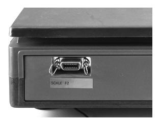
Figure 7-11. Remote Scale Channel Connector
