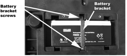
Figure 2-4. Removing Battery Bracket.
