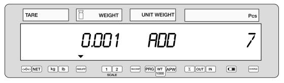
• Add exactly the number of pieces requested (the *PCS* display will go down to 0) and press the **PCS** key. The scale will compute and display the unit weight and the *INSUFF* lamp will go out.
