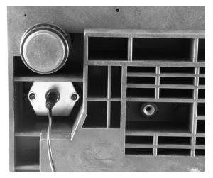
Figure 2-2. AC Plug-in Location on Underside of DC-788
