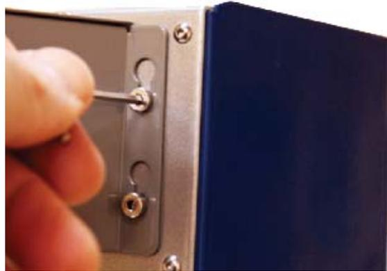
*Figure 2-10. Tighten Head Screws*
