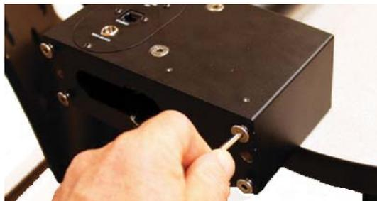
Figure 2-3. Remove Power Block Screws
