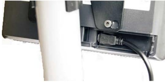
Figure 2-15. Insert Display Cable
