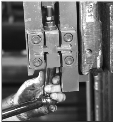
Figure 4-28. Remove Bottom Nut
