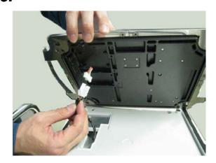
**7.** When running the cable, make sure to get it through the storage hole of the main unit.
