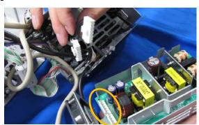
CAUTION: Here you need to disassemble the main board unit to unplug the FAN cable installed on the power board.
