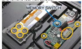
6. Detach the load cell and scale board P-1111A. Unsolder five wires to detach the P-1111A.
