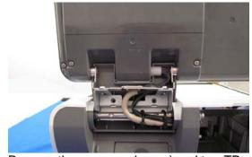
Remove three screws (green) and two TP screws (blue).
