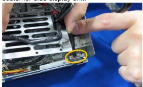
Unplug the connector (XJ13) connected to the power board.
