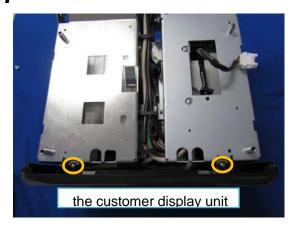
**2** Disengage three hooks located on the bottom of the main unit.
