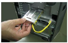
▼ Install the antenna jack (the jack connected with the white cable) on the antenna cover plate.
