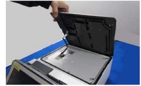
Attach two frames to the bottom of the platter.
