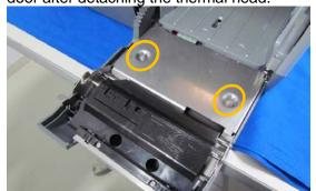
**3.** Remove the screw located on the bottom of the main unit.
