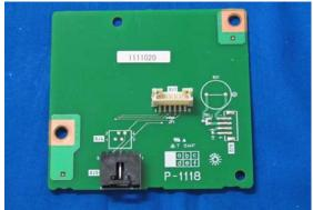
**9.** Detach the plate on which the relay board is installed.
