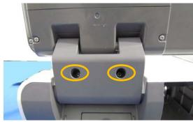
Hold down the display to detach the hinge cover (upper).
