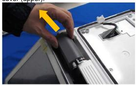
**7** Displace the main unit cover rightward to disengage the hook from the plate.
