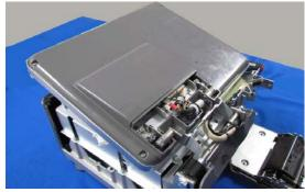
**4** Loosen two screws securing the hinge to detach the display unit.
