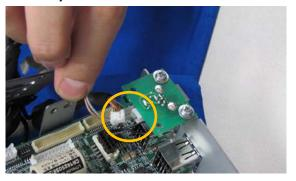
4-8 **UNI-9 Service Manual**  **26.** Detach the main board (remove the screws and detach the frame).
