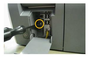
**2** Attach the antitheft cover for the USB flash drives and tighten the screw to secure the cover.
