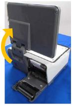
**3.** Remove two screws securing the hinge.
