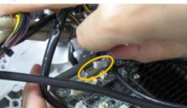
**21.** Unplug the connector (XJ12) connected to the speaker.
