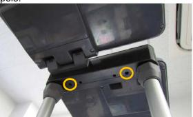
**3.** Remove two screws securing the hinge cover located on the back of the customer-side display.
