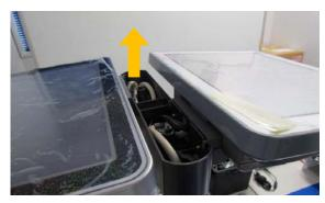
**4.** Detach the hinge cover located on the back of the customer-side display.
