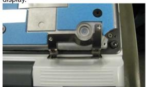
**2** Tighten two screws supplied with the kit to secure the guide platter.
