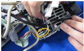
Unplug the connector (XJ21) connected to the peel-off sensor, label sensor and cassette sensor.
