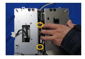
**3.** Disengage four clamps securing the cable.
