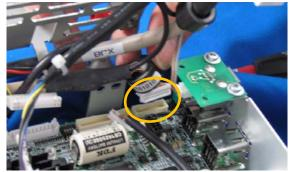
**25.** Unplug the connector connected to the modular jack board.
