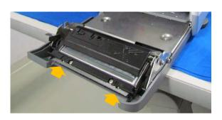
Note: If necessary use the two 1.5mm allen head set screws to adjust the thermal head alignment for optimal printing.
