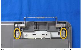
11 Remove six screws securing the display cover.
