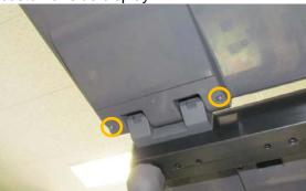
**5.** Detach the hinge cover (upper) located on the top of the pole.
