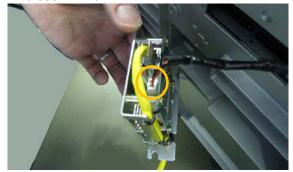
6. Tighten two screws to secure the wireless LAN unit.
