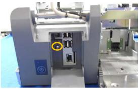
**4** Unplug the connector connected to the power switch board.
