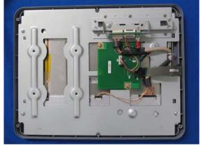
Unplug the connector (XJ1) and remove two screws.
