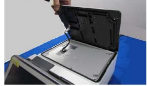
**4** Tighten four screws to attach the main unit cover supplied with the kit.
