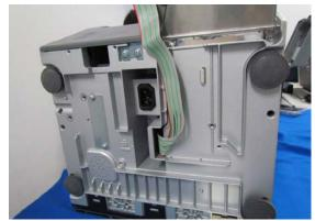
The thermal head cable is connected to the connector (XJ17) on the main board.
