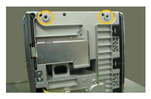
2. Hold the converter stand between the level adjusting feet and the bottom panel of the main unit to secure the stand.
