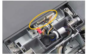
**7.** Remove four screws securing the hinge.
