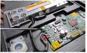
CAUTION: When installing the load cell, make sure to install it in the center of the
