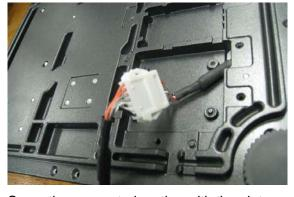
**8.** Cover the connected portion with the plate and tighten four screws to secure the plate.
