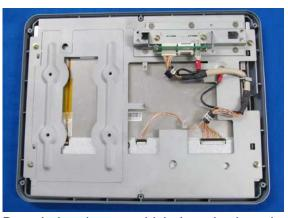
**14.** Detach the plate on which the relay board is installed.
