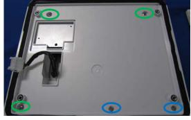
**8.** Open the left side of the main unit cover with the flat-blade screwdriver, etc.
