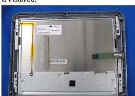
**8.** Remove two connectors and four screws.
