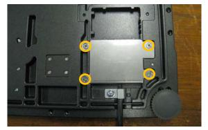
**UNI-9 Service Manual** 5-3 **9.**Connect the scale cable to the connector located on the bottom of the main unit.
