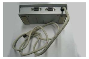
**2.** Run the cable along the guide on the bottom of the main unit to prevent the cable from being messed up.
