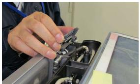
**2.** Detach the cover located on the top of the pole.
