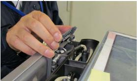
**2.** Detach the hinge cover located on the back of the operation display.
