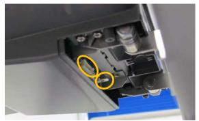
**9.** Remove four screws securing the hinge.
