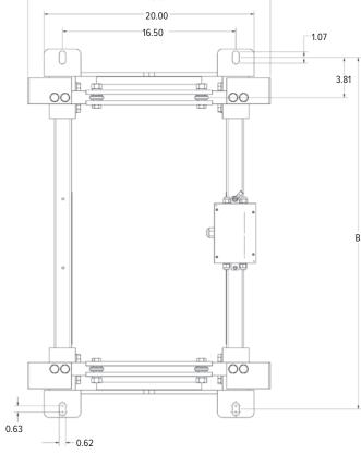
Note: Cables on drawings removed for clarity. Idler mounting hardware is not included in weigh frame; see idler mounting bolts above.
