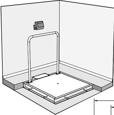
Image illustrates pit frame exposed to show detail.
