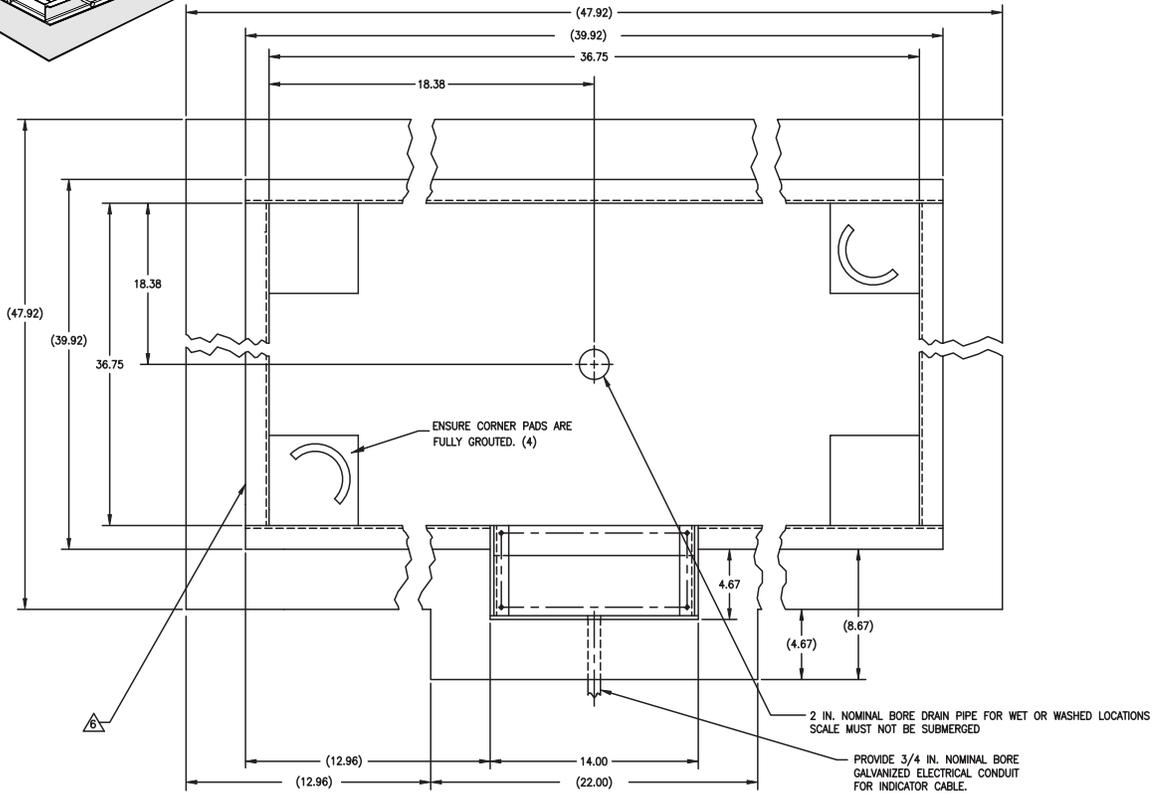
NOTE: HANDRAIL ON SCALE WILL MOUNT ON SAME SIDE AS JUNCTION BOX POCKET
