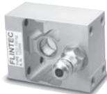
This high-accuracy stainless steel, single-point load cell is an ideal replacement cell for hopper applications with damaged bellows. This cell also features complete hermetic sealing for use in the toughest environments. This product is offered at 150 kg and comes complete with 10 ft of load cell cable.
