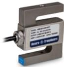
A stainless steel S-beam type load cell with trimmed outputs for easy installation. Compact and economical design, ideally suited for scale conversions and general-purpose weighing. NTEP Certified capacities range from 100 lb to 10,000 lb; non-NTEP Certified capacity of 50 lb, 15,000 lb and 20,000 lb. Complete with 20 ft of load cell cable. Trimmed outputs makes installation easy.
