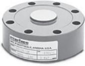
Resistance to extraneous forces allows for high fatigue life, less stringent mounting alignment and lesser possibility of reading errors. This design permits smaller, portable and compact testing machines. Capacities range from 1,000 lb to 100,000 lb. Complete with 10 ft of load cell cable.
