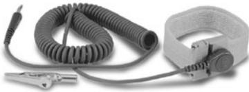
The single most important personal accessory for protecting ESD sensitive components and circuits, this wrist strap protects against charges from the body. The wrist strap consists of a comfortable elastic cuff or band and a detachable conductive cord for grounding the wrist band.
