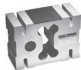
Single-point load cell featuring individual adjustment to eliminate corner errors and direct mounting of low-profile platforms to simplify the construction of floor scales, weigh bars, hanging scales and other types of weighing devices. High capacity range from 1,000 kg to 2,000 kg.
