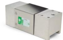
Low-profile, off-center loading load cell. Designed for direct mounting of a weighing platform and hanging scales. Long-term stability and durability are maintained. Capacities range from 100 kg to 500 kg. Complete with 3 m of load cell cable.
