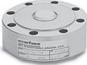
Designed specifically for difficult applications in harsh environments, these units incorporate welded stainless steel diaphragms to resist corrosion and seal against moisture intrusion. These load cells provide high accuracy, resistance to off-center loads with minimum error, excellent temperature specifications and low height envelope for ease of installation. Capacities range from 5,000 lb to 100,000 lb. Complete with 20 ft of load cell cable.
