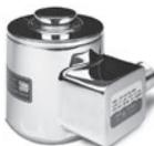
This welded-seal, stainless steel canister cell is designed for compression service only. High-capacity transducers are built for reliability, durability and extreme precision. Ideal for applications where ultimate precision is needed. NTEP Certified capacities range from 25,000 lb to 200,000 lb.
