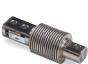
Hermetically sealed with an IP68/IP69K rating, this stainless steel, single-ended beam load cell has NTEP Certified for capacities from 5 kg to 500 kg. Comes with 3 m of cable.
