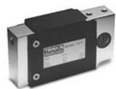
Off-center loading load cell designed for direct mounting of a weighing platform and simplified construction of platform scales. Long-term stability and durability are maintained. Load cells with potted cavities are available for improved performance in damp environments. The model 1015 has a balanced bridge for applications where multiple cells are used. Capacities range from 3 to 90 kg.
