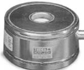
Bending ring load cell with low profile design ideal for high capacity weighing applications, including weighbridges, tanks, silos, high capacity platform scales and force measurement. Capacities from 5,000 kg to 30,000 kg and are OIML approved.
