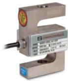
Suitable for single- or multiple-cell tension load applications. Nickel plated, high-alloy steel construction. Complete with 20 ft of load cell cable and full environmental protection with stainless steel side plates. Capacities range from 25 to 20,000 lb. Capacities of 5,000 lb or higher have standardized output for multiple-cell installations.
