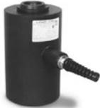
Single-column, environmentally protected design provides low deflection and trouble-free operation. High-alloy steel and epoxy coated construction yields reliable performance in harsh environments. Designed for high-capacity tension applications. Capacities of 20,000 lb and 50,000 lb. Complete with 35 ft of load cell cable.
