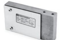
Designed as a replacement for the NCI® Mark III in hostile environments. Stainless steel, moisture-resistant single-point cell. Complete with 10 ft of load cell cable. 10 lb to 25 lb cells may be used with a base size of 8 × 8 inch; 50 to 200 lb cells may be used with a base size of 12 × 12 inch.
