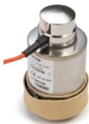
A rocker column load cell specifically designed for high-capacity weighing in the harshest environments. Ideal for truck scale applications, it features all stainless steel construction with IP68 hermetic sealing. Easy to install and maintain. Available in capacities ranging from 20 t to 60 t and includes 12 m of load cell cable.
