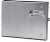
Very high-performance single-point cell designed for high-precision counter scales. Resistant to moisture and severe impact loading. Capacities range from 2 lb to 250 lb. Complete with 10 ft of load cell cable.
