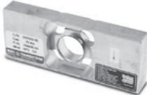
This stainless steel, welded-seal, low-profile single-point load cell is designed for bench scale and checkweigher applications in caustic/acidic environments. Insensitive to off-center loading and tolerates most severe washdowns. Comes complete with 10 ft of load cell cable.
