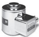
This welded-seal, canister cell is designed for compression service only. High-capacity transducers are built for reliability, durability and extreme precision. Compression Precision (CP) cells are recommended for most industrial applications. Single bridge available for 10,000 lb to 500,000 lb capacities, dual bridges available upon request. Complete with 30 ft of load cell cable.
