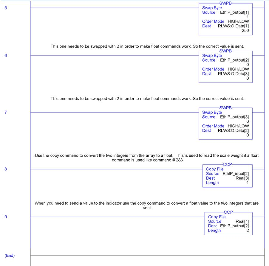
Figure 3-6. Ladder Logic for EtherNet/IP
