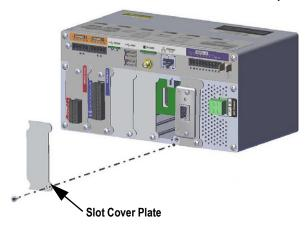
Figure 2-3. Existing Cover Plate Removal
