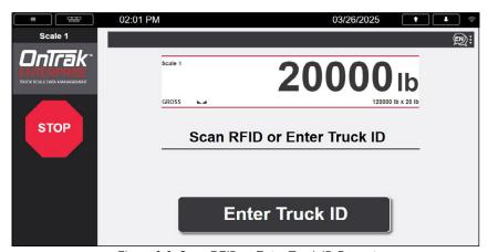
Figure 2-3. Scan RFID or Enter Truck ID Prompt
