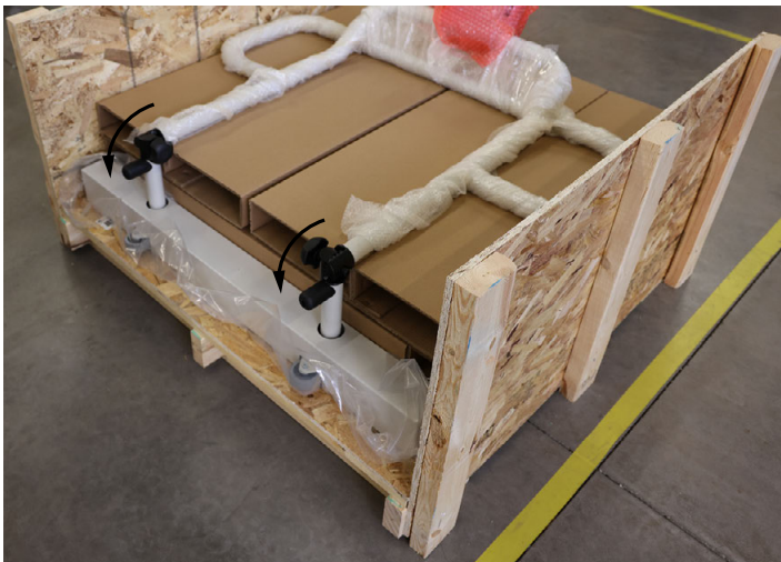
Figure 2-5. Raising Handrail and Removing Cardboard Platforms
