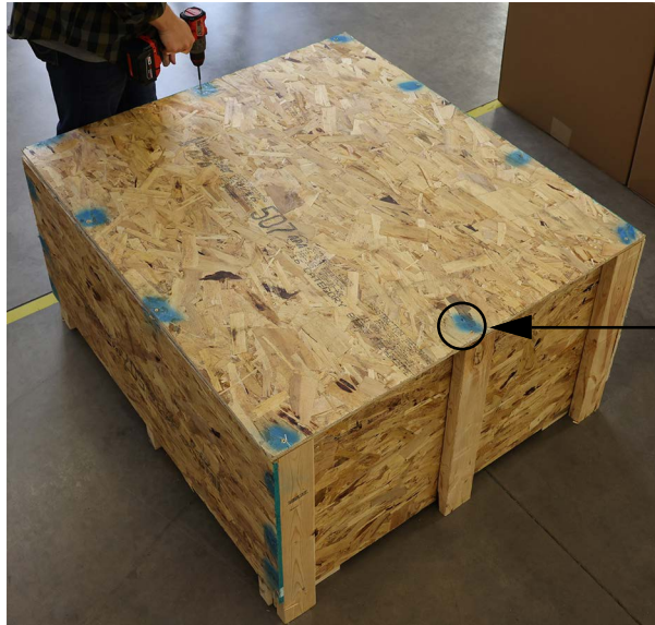
Figure 2-1. Crate Cover Screw Removal
