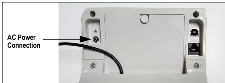
Figure 2-15. Power Connection Site
