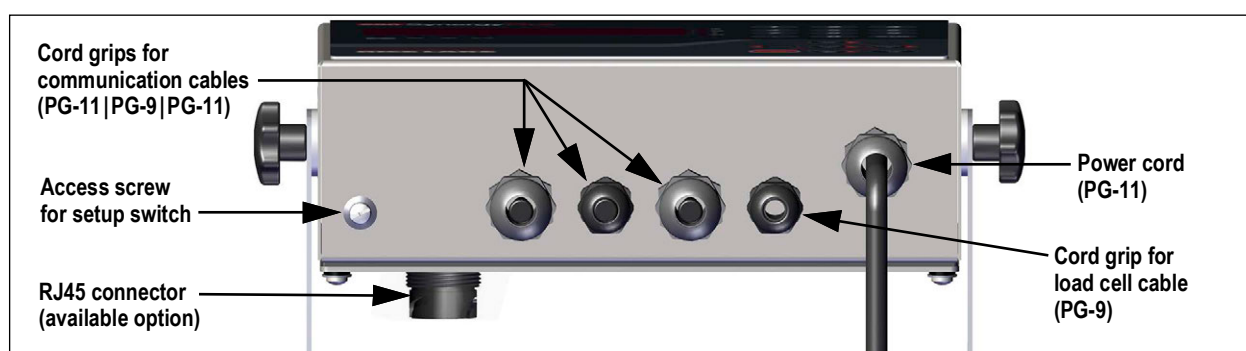
Figure 2-5. Recommended Cord Grip Assignments
