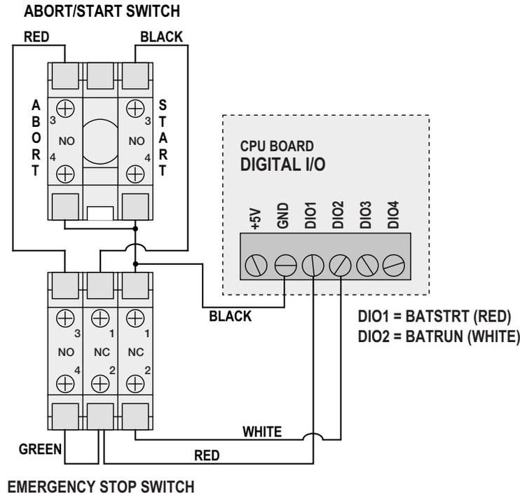
Figure 14-2. Batching Switch and Wiring Diagram Example
