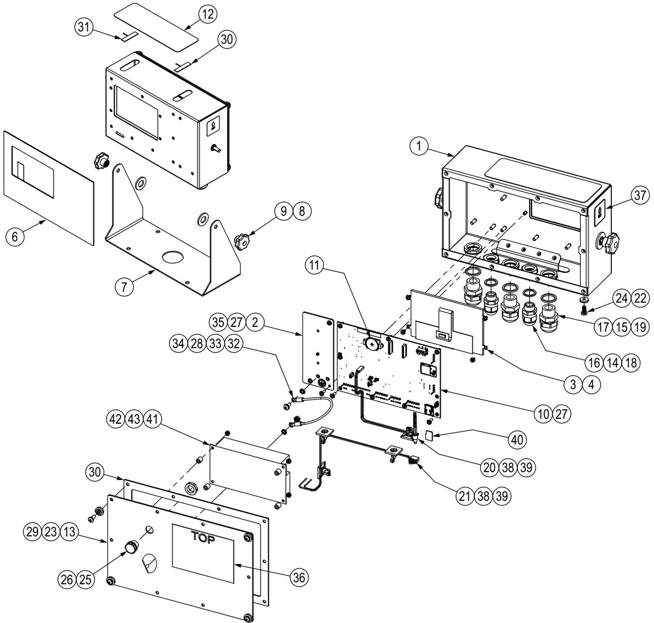
Figure 2-14. 682 DC Models Replacement Parts Diagram
