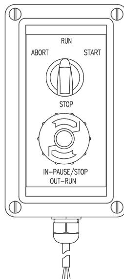
Figure 14-1. Batching Switch
