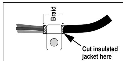
Figure 2-7. Braid Shielded Cable
