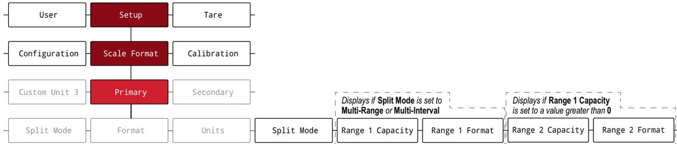
Figure 5-1. Setup – Scale Format Menu – Split Mode
