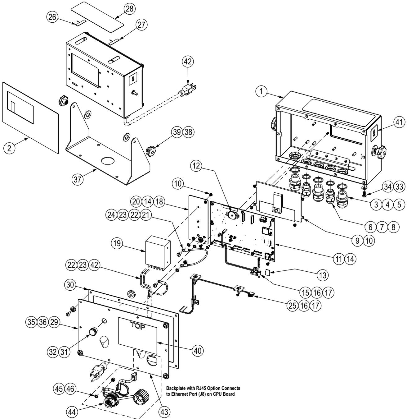
Figure 2-13. 682 AC Models Replacement Parts Diagram
