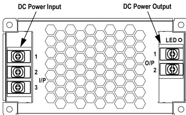
Figure 2-9. DC Power Supply Board (PN 209417)
