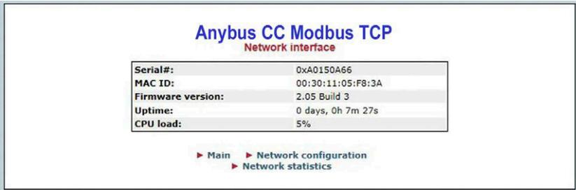
Figure 3-5. Modbus TCP Network Interface Display in a Web Browser
