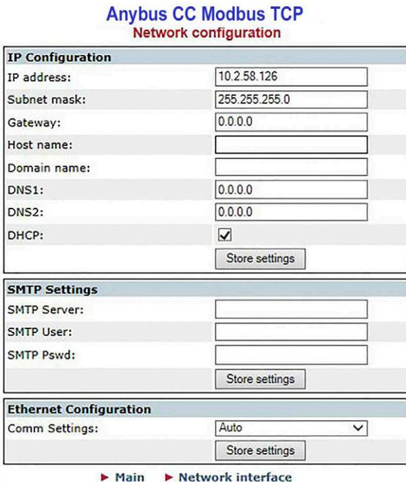
Figure 3-6. Modbus TCP Network Configuration Display in a Web Browser
