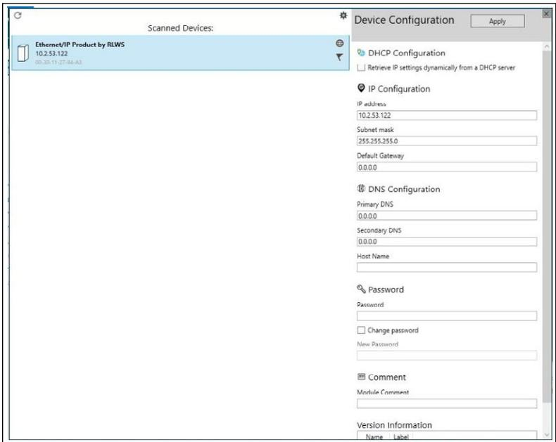
Figure 3-3. IP Configuration Utility - Enter Network Settings
