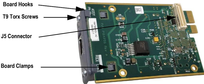
Figure 2-3. Bottom of Carrier Card with Module Installed
