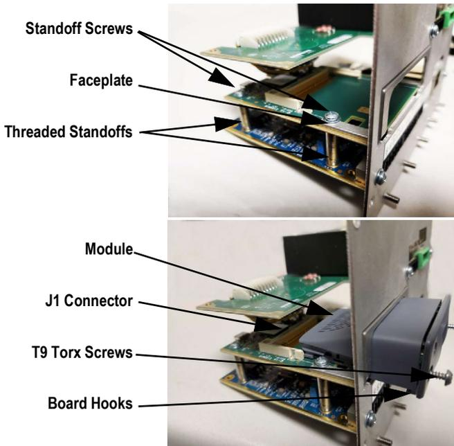
Figure 2-4. 880 Panel Mount Interface Option Card Installation
