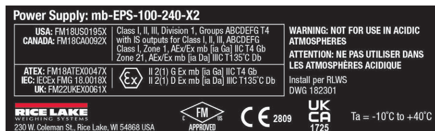
Figure 3. mb-EPS-100-240-X2 Power Supply Label
