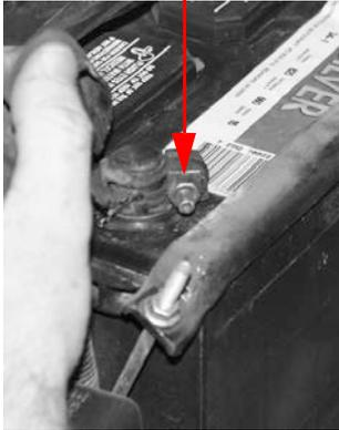
Place wire on cable clamp stud and secure with nut.
