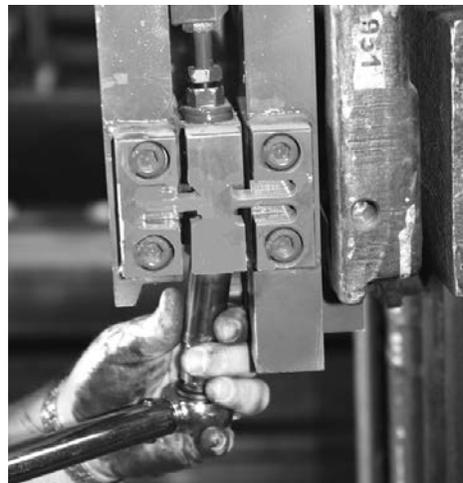
Figure 6-13. Tightening the Lower Hex Nut
