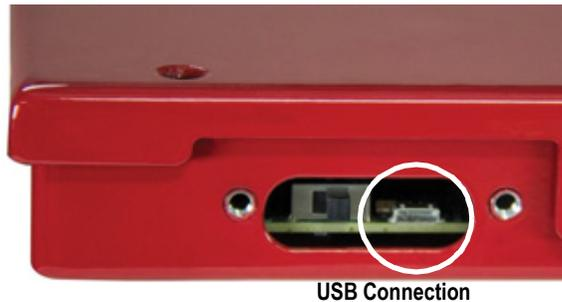
Figure 4-23. Micro B USB iQube2 Junction Box Connection
