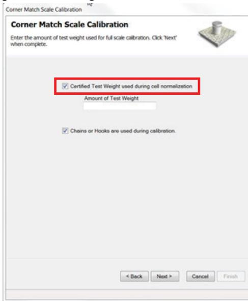
Figure 5-28. Certified Test Weight Used During Cell Normalization Checked
