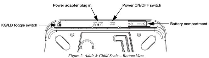
5. Use the **POWER ON/OFF** toggle switch located on the underside of the scale to activate the scale.
