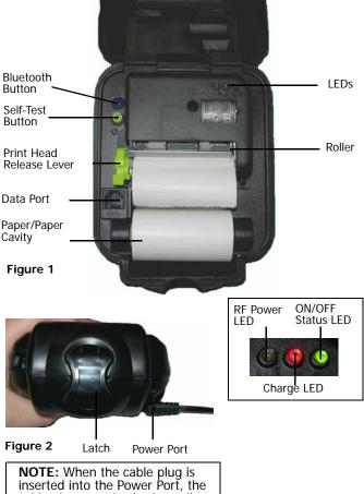
**NOTE:** When the cable plug is inserted into the Power Port, the cable plug must lay horizontally to the bottom of the surface of the case.
