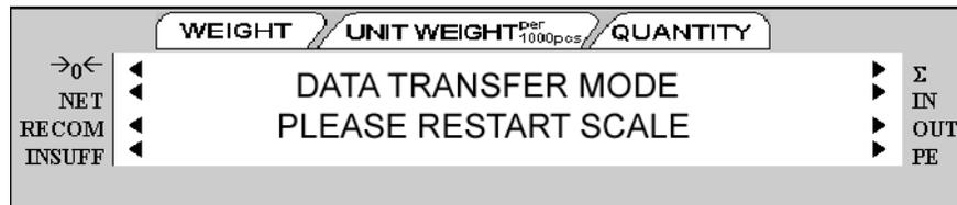
Turn the scale off and then on again, using the on/off switch located on the bottom of the scale at the back.
