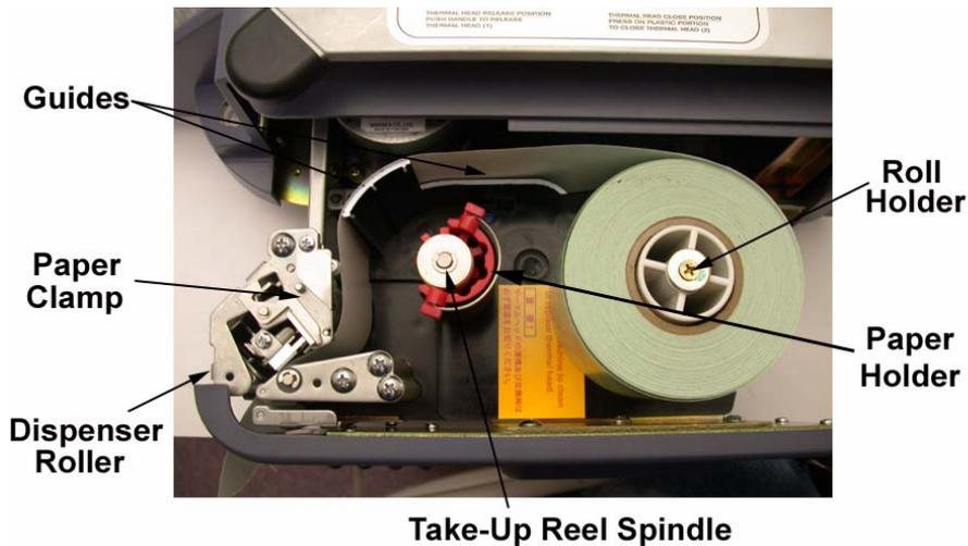
Figure 7-20. Loading DC-300 Printer
