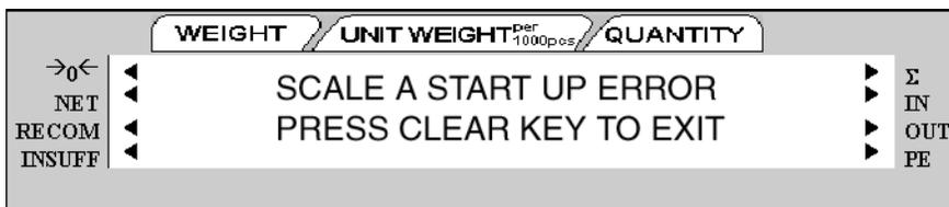
Remove the weight from the platform and press the **CLEAR** key to exit.
