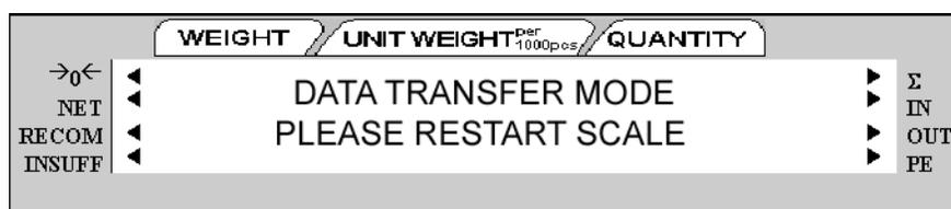
The scale should be powered down and then powered back up to initialize the new changes. When the scale is powered back up, it will still be in the *DATA TRANSFER MODE - READY* state. To exit the Data Transfer Mode, continue with the instructions below.
