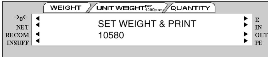
The display confirms that the span settings for calibration of the scale are being saved
