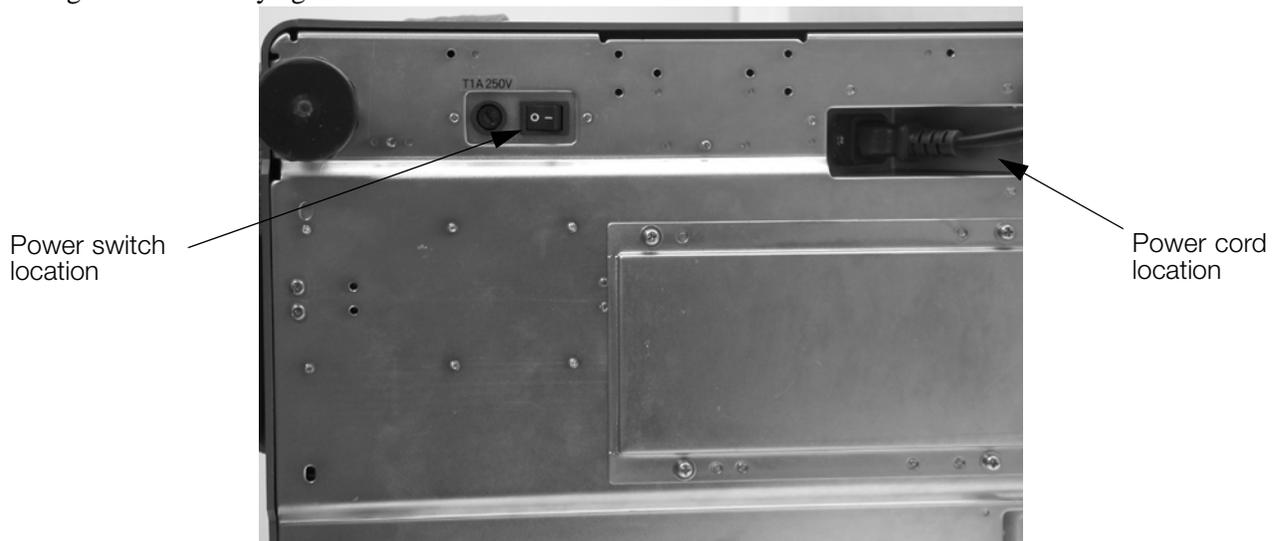
Figure 2-3. Power Switch and Power Cord Location
