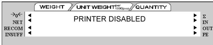
Pressing the \* REPRINT key while holding down the REZERO key again will re-enable the built-in printer, showing the following on the display:
