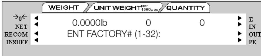
2. From the numeric keypad, enter the number of the Factory Name you want to be active for label printing, then press the \* **REPRINT** key.
