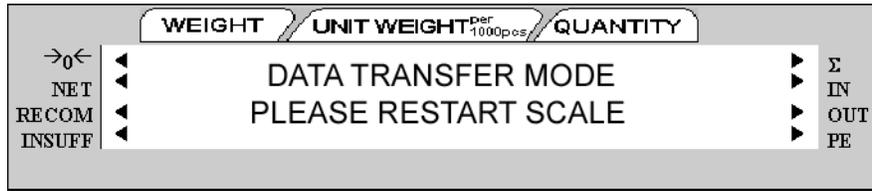
Turn the scale off and then on again, using the on/off switch located on the bottom of the scale at the back.
