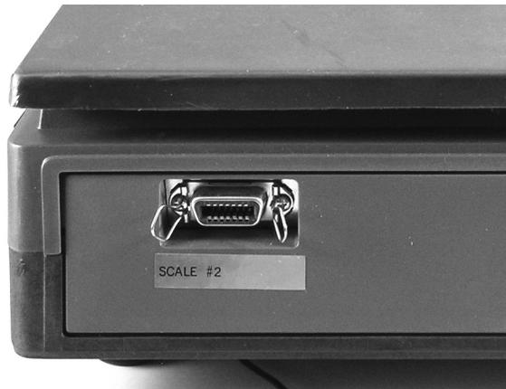
Figure 7-11. Remote Scale Channel Connector
