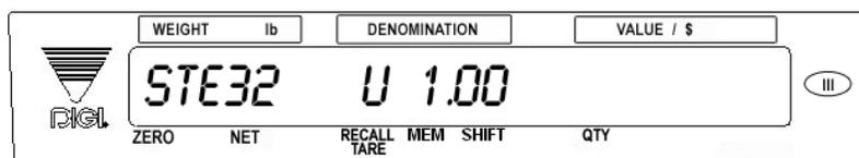
2. After a test of the different elements of the display, the scale takes you to the stand-by screen in the Weighing Mode. SPEC 20, Bit 2 - Selection of Segment-Check Style controls whether the startup test of the segments is Fast or Standard. At the stand-by screen the *WEIGHT*, *DENOMINATION*, and *VALUE* displays show zeroes.
