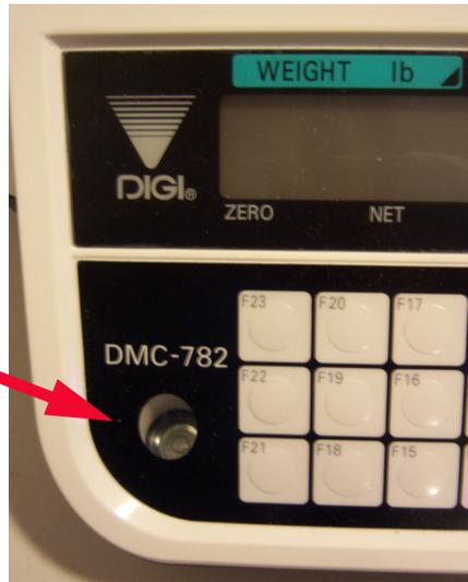
Figure 2-1. Leveling Bubble
