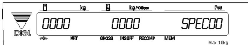
The *VALUE/\$* display shows what specification you are in (in this case, SPEC00). The *Denomination* display shows how this specification is currently programmed (Bit 3 = 0; Bit 2 = 0; Bit 1 = 0, and Bit 0 = 0 in this example, while the *Weight* display will show any changes you enter.
