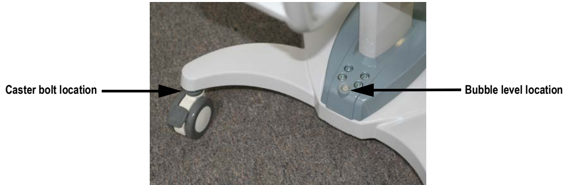
Figure 2-14. Bubble Indicates That The Scale is Level
