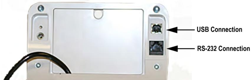
Figure 4-1. Connection Ports
