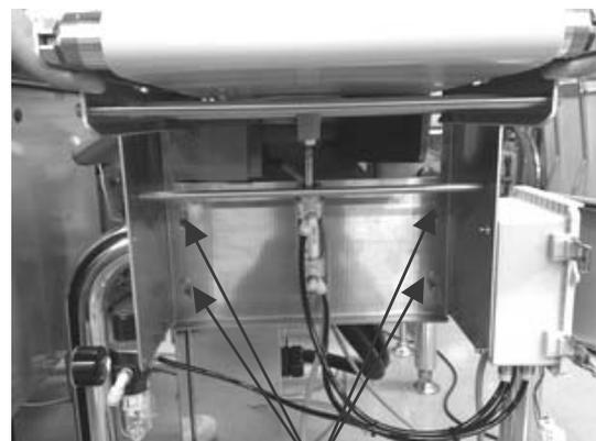
Loosen the screws to adjust the conveyor height.
