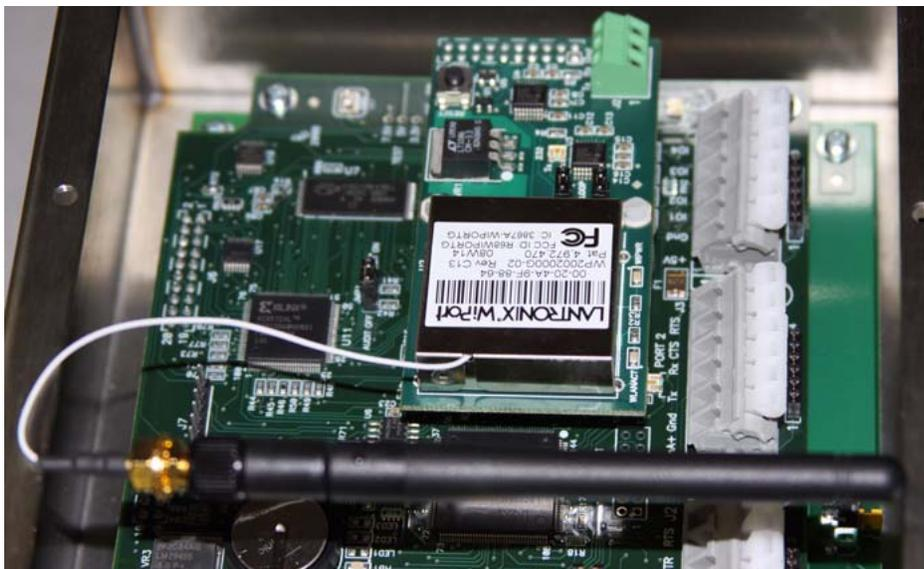
Figure 4-2. Antenna installed on card
