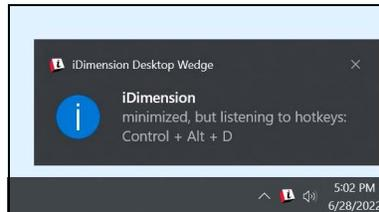
2. Click ^ in the notification area of the taskbar to open the system tray and select the iDimension icon to display the iDimension Desktop Wedge application.
