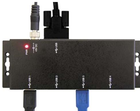
Figure 2-8. FTDI USB to Serial Converter Connection
