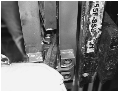
Figure 6-13. Centering the Load Cell Using a Chisel
