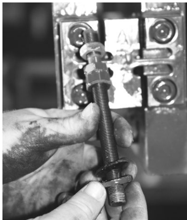
Figure 6-5. Remove Flexure Rod with Nuts and Washers
