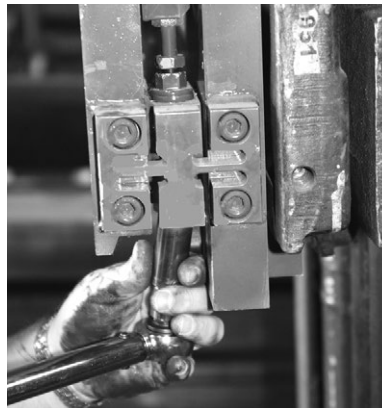
Figure 6-14. Tightening the Lower Hex Nut
