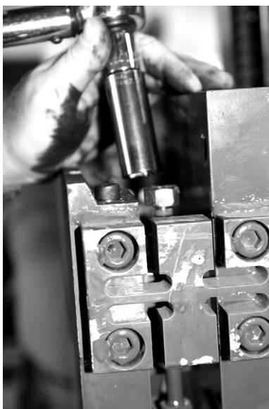
Figure 6-3. Removal of Hex Nut (#1 of Parts Breakdown)
