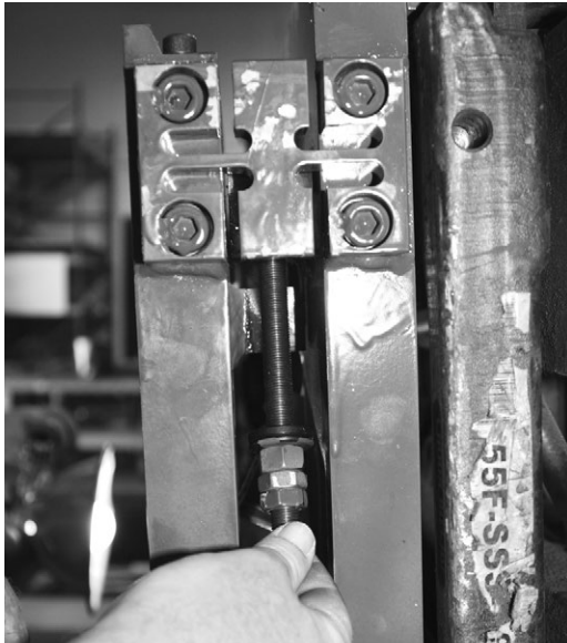
Figure 6-9. Installing Flexure into Scale
